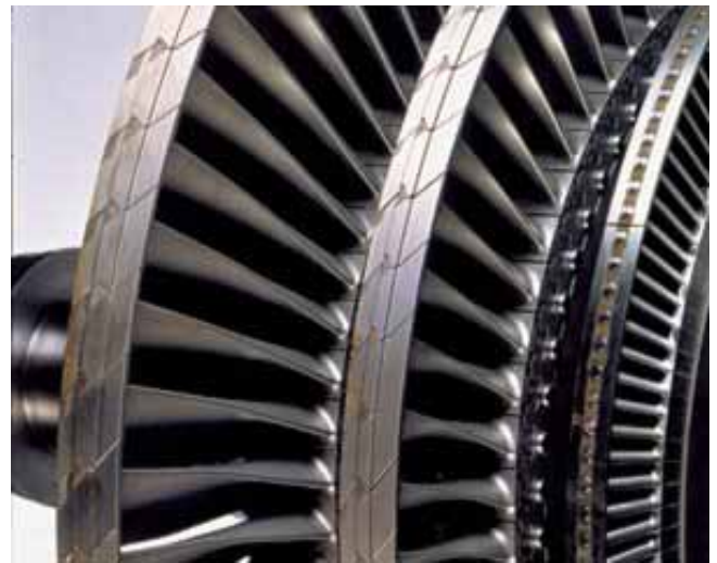
Exposed Steam Turbine Rotor
